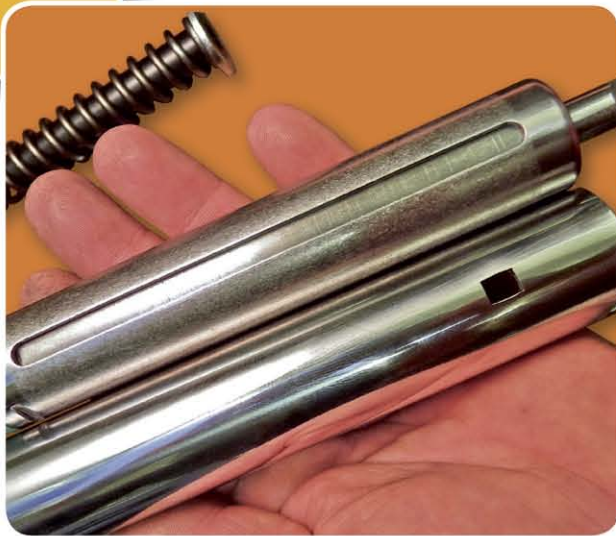
Above: The piston (top), showing the fitted piston sleeve
